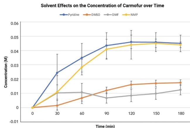
Figure 4. Concentration of carmofur over time with various solvents. NMP was found to have comparable yields as pyridine, which has enabled more convenient scale-up of carmofur and its related analogs.
