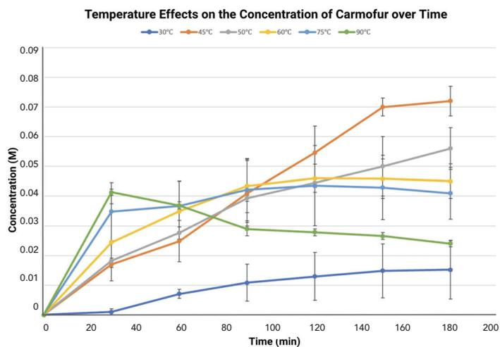
Figure 2. Concentration of carmofur over time with various temperatures in pyridine. 45 °C was found to be the optimal temperature.
