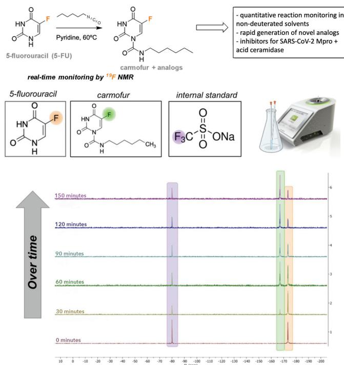
**Figure 1.** A time course is generated through kinetic monitoring by  $^{19}F$  NMR spectroscopy, where real-time formation of carmofur can be observed.
