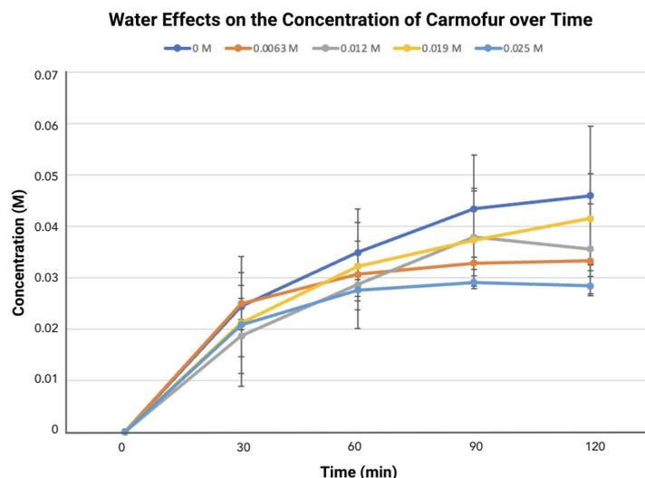
Figure 3. Concentration of carmofur over time with increased concentrations of water in the reaction.
