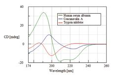
CD spectra of Human Serum Albumin (Helix rich), Concanavalin A ( $\beta$ -sheet rich) and Trypsin inhibitor (Random rich) in water with excellent signal to noise to 174 nm.
