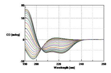
Above: 2D-CD Spectra of sodium poly-L-glutamate titrated with diluted sulfuric acid.
