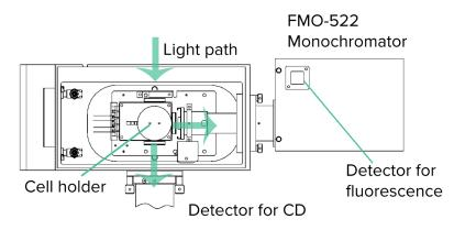
Above: Configuration for emission scanning with FMO-522
