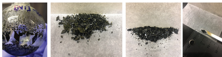
Figure 1. Ni(II) Schiff base complexes prepared in this work. From left to right: large crystals grown from a solution of 1 in chloroform and hexanes; recrystallized complex 1 ; recrystallized complex 2 ; isolated crystal of 1 , demonstrating the ease with which large crystals of these complexes can be grown and isolated.
