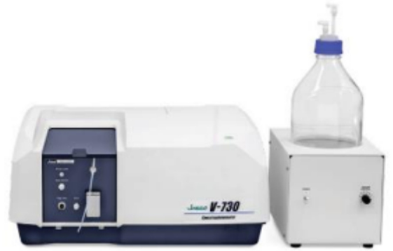
UV-Visible spectrophotometer equipped with a vacuum sipper
