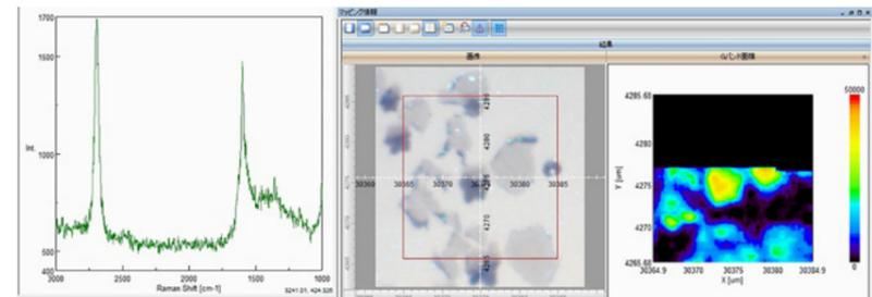
QRI Imaging with EMCCD, high speed stage and digital filtration
